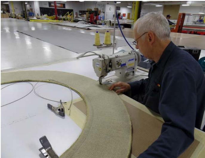
Zetex®, ZetexPlus®, and Z-Block™ Steel™ wire reinforced fabrics are commonly used to make fabric expansion joints. The wire ensures that the expansion joints remain in tact despite being subject to repetitive movement.
